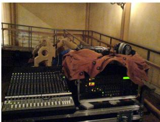
**Signal chain**: All microphones into separate channels on Mackie ONYX 1604, analog signal from there to Tascam MX2424 digital HDD multitrack. Backup from Mackie analog to portable Tascam DAT.
