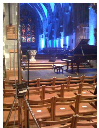
• Two Neumann KM140 condenser microphones, cardioid, mounted on stand at piano end, semicoincident and angled 90° apart, NRK style.
